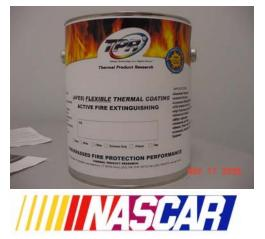
The environmentally friendly, water based coating is designed for and can be applied to the protective wall panels and foam being used in the new COT, debuting in March 2007. It is also effective at reducing heat soak on highly other plastics and components such as fiberglass, carbon fiber and other composites used widely in professional motorsports.
